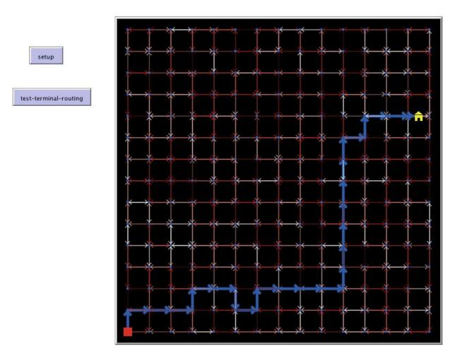
This image shows the interface of our code. When test-terminal-routing is clicked a link between the station node in the bottom left corner to the randomly generated incident node is created.
